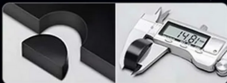
15mm black acrylic cutting in one-pass
